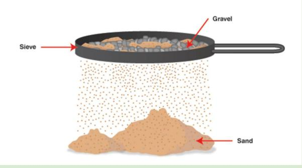
The process of sieving is when you pass a mixture of different solids through a fine mesh.
